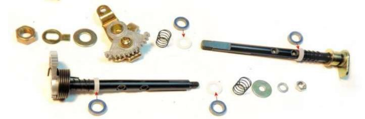
Bearings will freely slide onto the throttle shaft and will also fit the throttle shaft bore, both without any machining. It is recommended to clean the threads on the throttle shaft with an M4 tapping tool so that the new screws fit. These screws are designed to be smaller to have less air drag, they are made of stainless steel to have strength, and the threads are in top tolerance to hold well. They have a hollow end that can be stretched to hold in the thread.
