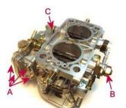
After removing the throttle valves unscrew all screws marked with the letter A. These screws can be loosened and it is not necessary to dismantle the pump. Loosen the nuts marked B and C and remove both throttle shafts. We recommend taking it out slowly and carefully and stacking everything as it belongs so you know the correct order later. All bushings will be replaced with bearings. The bushings in the photo are white, but can be black.
